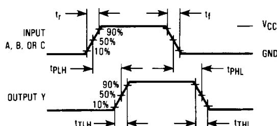
Figure 1. Switching Waveforms
